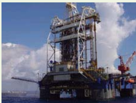
The deepwater drilling rig, Cajun Express , conducts the Jack No. 2 well test in the Gulf of Mexico.
