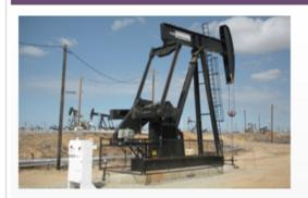
In California's San Joaquin Valley and elsewhere, CES has helped increase oil field pump performance by promoting adjustable speed drives, which save energy and also cut maintenance costs.
