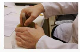
2. Grind and Mix Using a pestle to prevent contamination, a technician grinds the drill cuttings for mixing with a chemical solution that "digests" the powdered rock, creating a sample.
